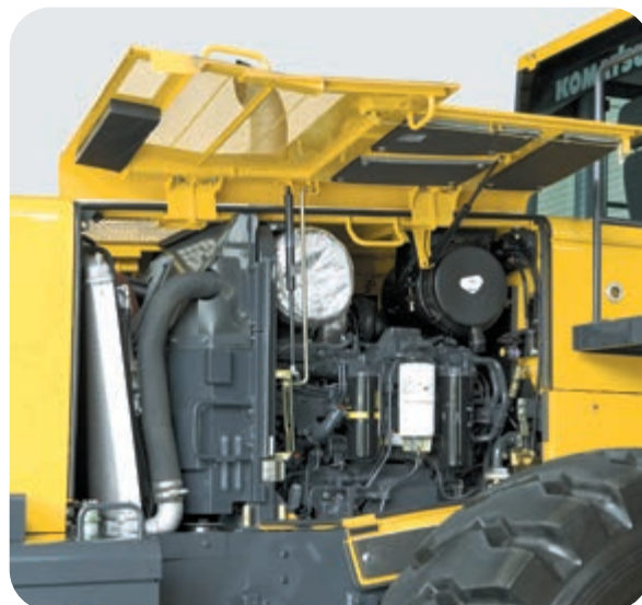
Gull-wing doors for easy ground level access
