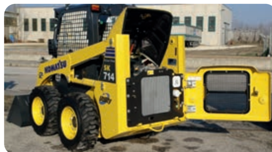
The hatchback: simple inspection and cleaning of the radiators
