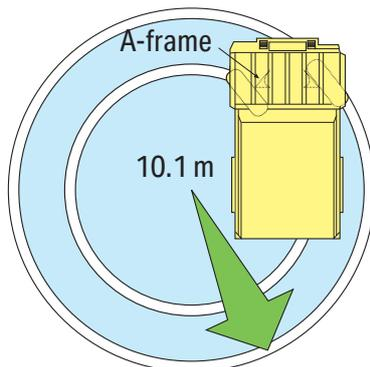
Turning radius varies depending on ground conditions and/or vehicle speed.
