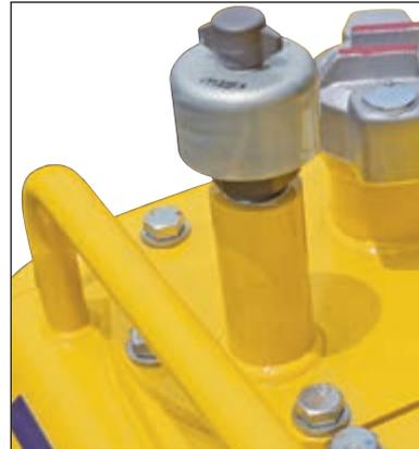
The fuel tank is equipped with a high-filtration breather with pressure valve to prevent dust from entering.
