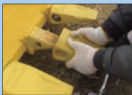
Set PAB tooth to horizontal pin type adapter
